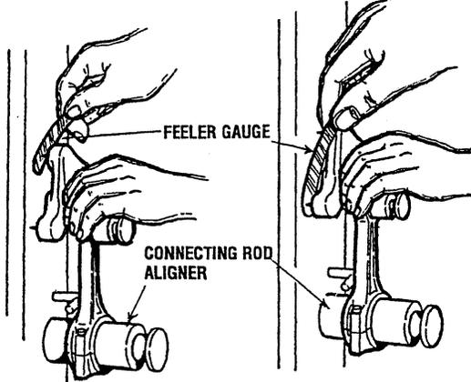
**CONNECTING ROD TWIST LIMIT** 0.004in (0.1mm)
