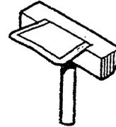
**CRANKSHAFT REAR OIL SEAL INSTALLER**
