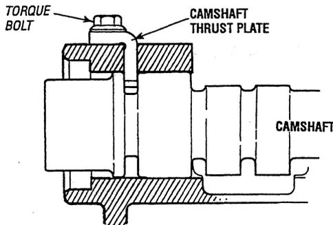
3. Measure the end play of the camshaft by inserting a feeler gauge in the gap between the rear of the thrust plate and the new front camshaft journal.
