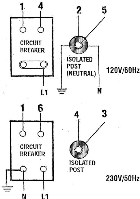
**NOTE:** Correctly position the case ground wire (white/green) onto the neutral/ground terminal.
