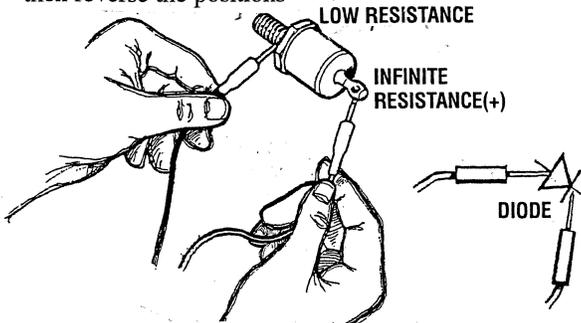
A low resistance should be found with the leads in one direction and infinite resistance (blocking) in the other direction.
