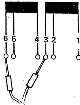
TEST EACH OF THE WINDING LEADS INDIVIDUALLY AS SHOWN
