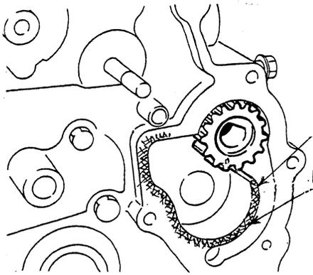
LOCKTITE #518 **MUST** BE APPLIED TO THE SHADED AREA TO ENSURE A PROPER SEAL
