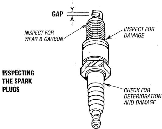
**NOTE:** Loctite Anti-Seize applied to the threaded portion of the spark plugs will retard corrosion, making future removal of the spark plugs easier.
