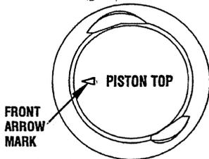
Securely pressing the piston ring with the ring band, insert the piston and connecting rod assembly into the cylinder. Keep in mind that the piston ring may be damaged if hit too strongly.
