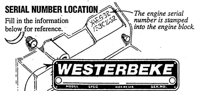
The engine model number and serial number are printed on a decal on the engine manifold.
