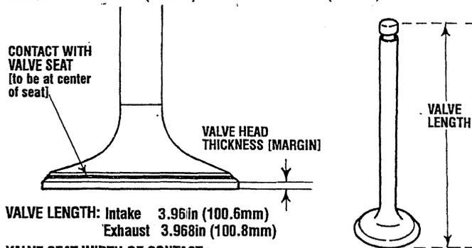
VALVE LENGTH: Intake 3.96in (100.6mm)
