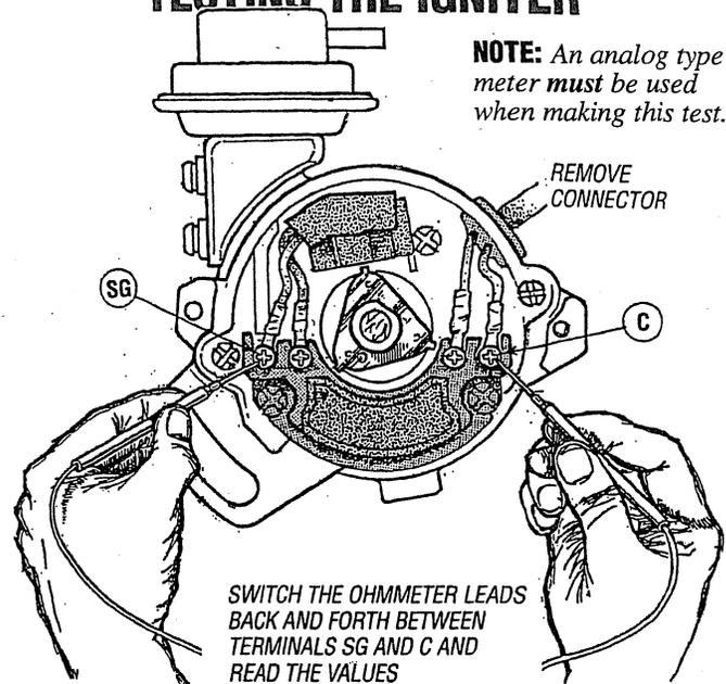
SWITCH THE OHMMETER LEADS BACK AND FORTH BETWEEN TERMINALS SG AND C AND READ THE VALUES
